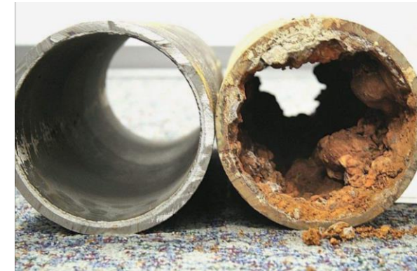
Cast Iron Pipe & Tuberculation
